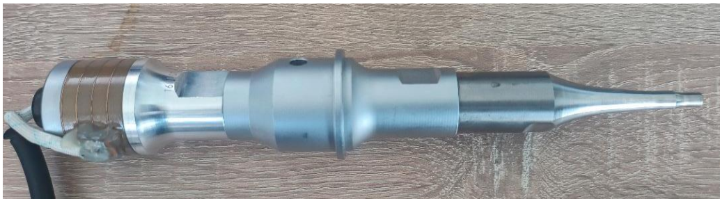
Fig. 5. Ultrasonic system designed for plastic and composite materials welding
